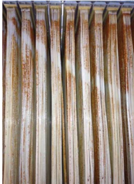
Figure 12. Electrostatic Particle Accumulation (ferric) on UF Elements
