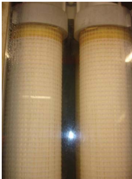
Figure 11. 20 ppm ACH With pH and Particle Charge Control With no Particulate Accumulation
