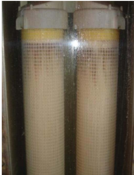
Figure 9. Precipitated Floc Particle Accumulation via “Electrostatic Attraction” With 20 ppm ACH
